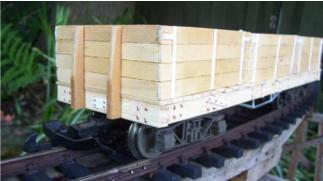
The floor and frame are slit pine, sole bars, buffer beams and planks before adding side gates and ends.
